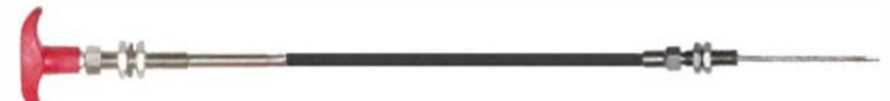
XLMRSC-LENGTH (Throttle / Fuel Shut off) Free Length: 175mm | Conduit: 7.0mm | Inner: 1.5 mm SS-Wire Rope
